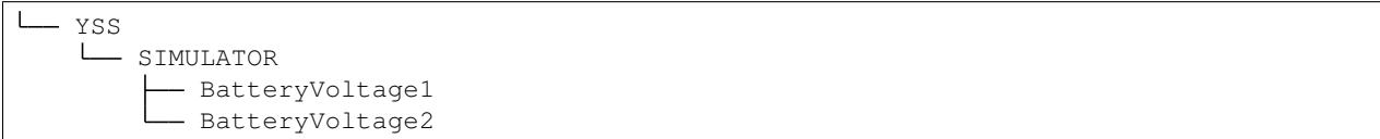
we find two space systems /YSS and /YSS/SIMULATOR and two parameter entries /YSS/SIMULATOR/BatteryVoltage1 and /YSS/SIMULATOR/BatteryVoltage2.
